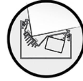
COVE / CORNICE LIGHTING
